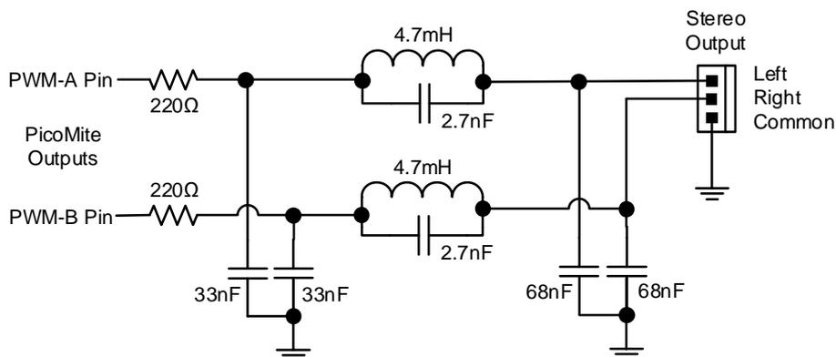
Both circuits are designed to feed an amplifier (not directly drive a headphone or speaker) and rely on capacitor coupling into the following amplifier (most have this).
