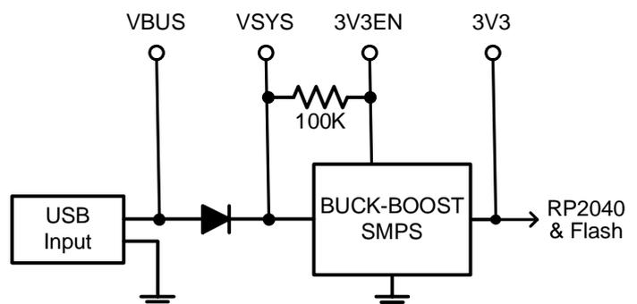
To minimize power supply noise, it is possible to ground 3V3EN to turn off the SMPS. When shutdown the converter will stop switching, internal control circuitry will be turned off and the load disconnected. You can then power the board via a 3.3V linear regulator feeding into the 3V3 pin.
