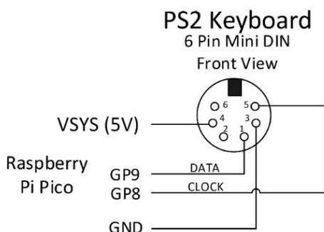
The I/O pins on the RP2350 series of microcontrollers can withstand 5V (while powered up) so the keyboard can be directly connected as illustrated with the 5V supplied by the VSYS pin on the Raspberry Pi Pico 2.
