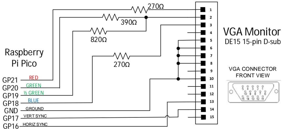
The output is in the standard VGA format with a pixel rate of 25.175MHz and a frame rate of 60Hz.
