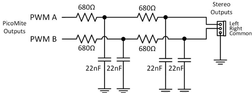
Below is a superior circuit producing quality audio with an insignificant amount of the carrier remaining. This is suitable for a more sophisticated HiFi amplifier/speaker configuration. The output is good for 10Hz to 15KHz at about 3V peak to peak (1V RMS) at 1KHz.
