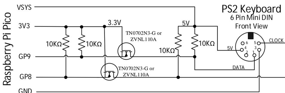
The recommended MOSFET is a TN0702N3-G or ZVNL110A however the commonly available 2N7000 has been tested and works well.
